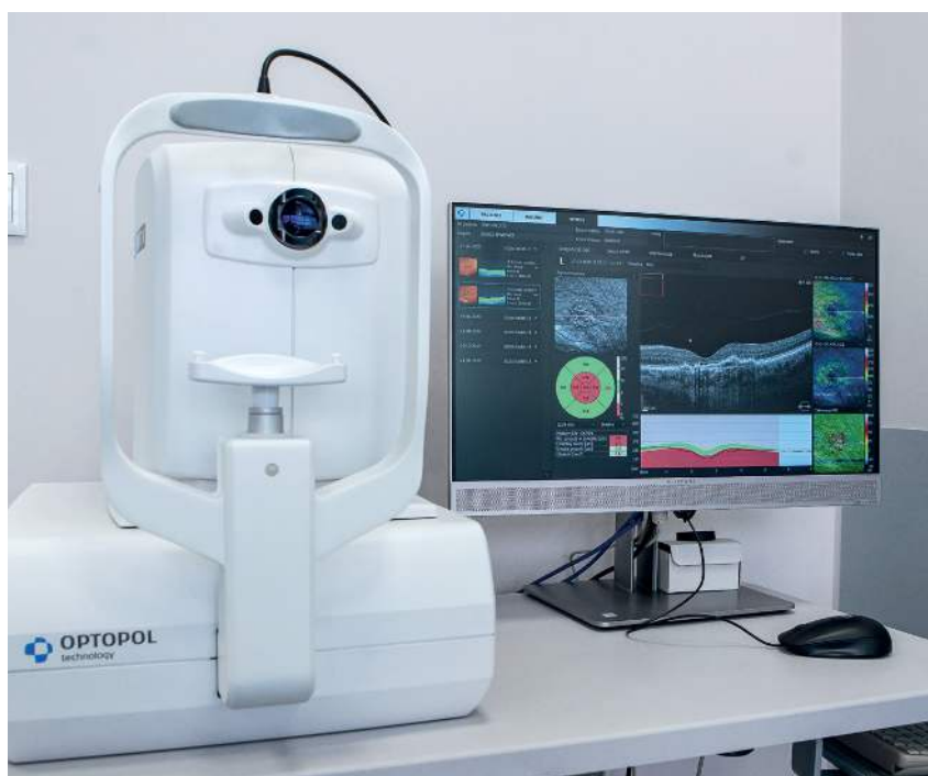
Figure 20. Retinal Spectral Optical Tomograph using Optopol's Revo system.
