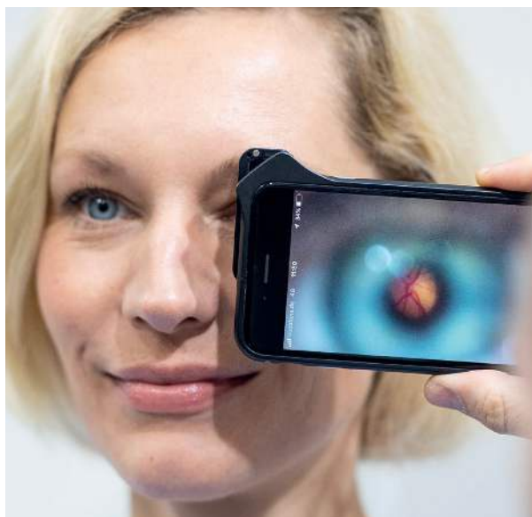
Figure 2. D-Eye – an example of an ophthalmoscope on a smartphone.
