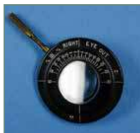
Fig.2 ► Risley's rotating prism, which can be inserted in the slot of a trial frame
