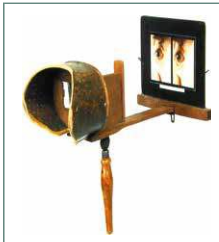
Fig.1 ► Holmes stereoscope (From Eye and Instruments by Isolde den Tonkelaar, Harold Henkes and Gijsbert van Leersum. Batavian Lion 1996)
