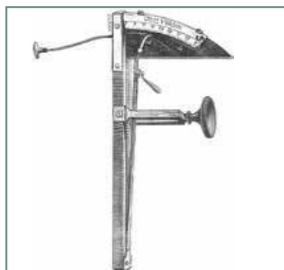
Fig.2 ► The Fick Oswalt ophthalmotonometer where a smoked glass plate was incorporated to facilitate reading of the pressure value
